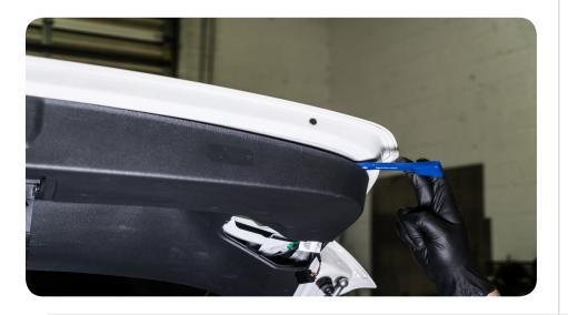
9. Once all plastic is removed, snake wires through pillar on both sides.
