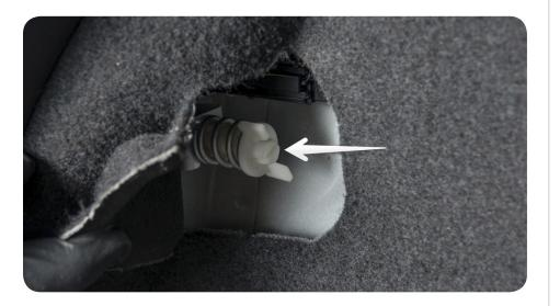
24. Plug PIN 1 (D1/P1) into wiring harness (SLOT 1). D1 + P1 are the same steps for each side of the car.
