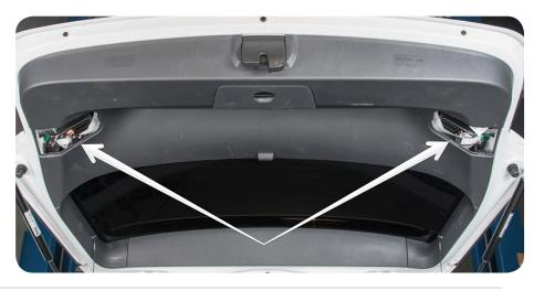
3. Locate connectors behind the hatch lights and push red clip to unlock (1). Then push down clip (2) and unplug the harness. Remove two 8mm nuts from rear of each light. Repeat for other side and unplug OEM harness.
