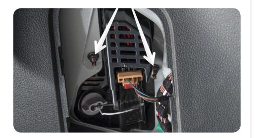
19a. Working from the other tail lights -- locate cut-out in rear panelling and pop open on both sides.
