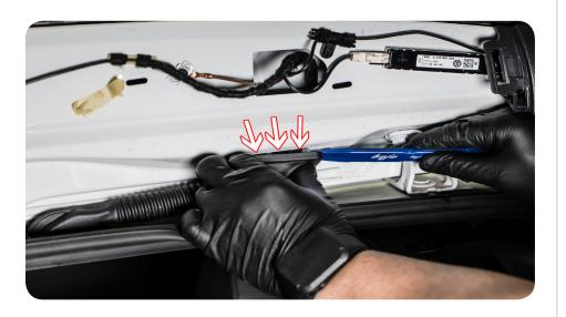
13. Attach outer tail light harness to snake through rubber tube. Be careful not to damage rubber tube. Repeat on both passenger + driver side (harness is labelled)
