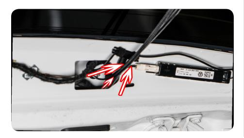
15. Use (8) zip ties to secure harness to factory wiring for tidiness on both sides + quide and zip tie both side harnesses towards the inner light mounting locations.
