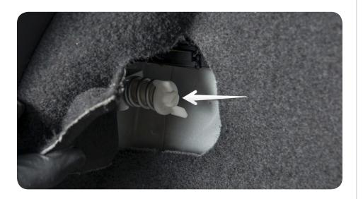
20. Release red clip + remove tail lights just enough to reach the OEM plug between the lights and the car.
