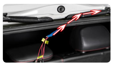
14. Feed wires that you routed in the rubber tube through the top of hatch opening along column (for outer tail lights)
