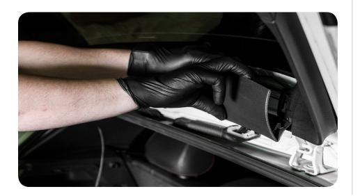
7. Remove (4) T20 screws from back hatch
