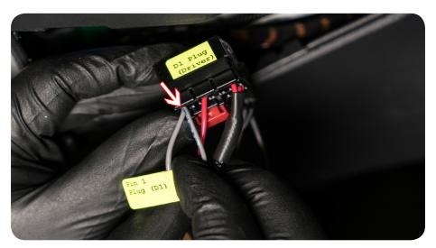
25. Plug PIN 5 into SLOT 5 (D1/P1) and push the locking tab back in.
