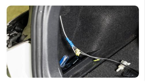
11. Feed taped wires through side pillars towards the middle of the roof.
