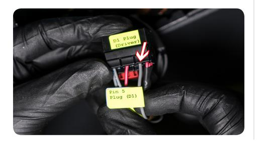
26. Use the wire in the previous step labeled "Plug D1/P1 - T-Tap", and insert the wire through the hole on the t-tap. Shut the t-tap to a click to make sure it is secure.
