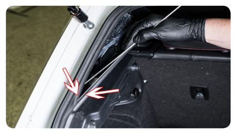
10. Thoroughly tape wires to snake through opening. One one side is completed, do the same thing for the other side.
