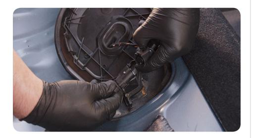
5. Connect both ends of the D-Connector into their respected slot on the Burnout Box. Then tuck away into the panel and close back up. Reinstall the seat and plastic covers and then your all done!
