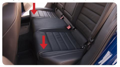
2b. To remove the rear seat pull the bench straight up in the areas indicated in step 2a. If the seat is being difficult to remove try pulling back on the seat while you lift upwards.
