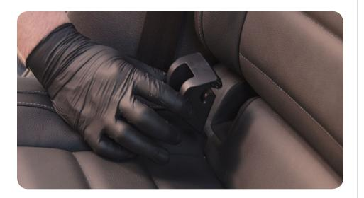
2a. \*Seat removal demonstrated is on a MK7 Golf R, the process is very similar on most Volkswagen and Audi Models. To remove the seat you must release the two retaining clips located in the areas marked below. (Next step on how to remove)
