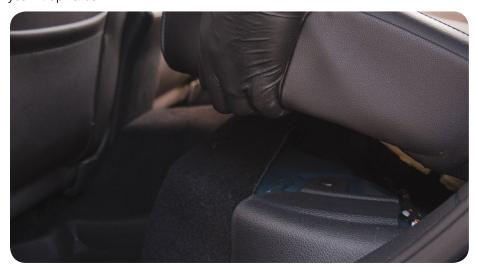
3. Locate the plastic panel on the driver's side and remove by simultaneously pushing forward and pulling upwards on the bottom of the panel, revealing the D-Connector.
