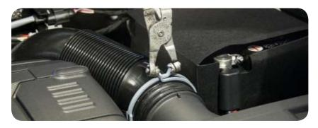
6. Grasp the factory air box and remove by pulling up.
