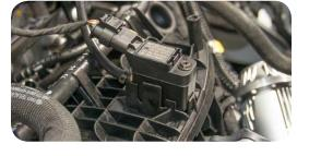
20. Route the included vacuum hose from the boost tap to the blow off valve. Secure with the include zip ties.
