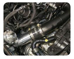
13. Install the upper outlet pipe into the coupler at the turbocharger. Install the lower outlet pipe from the top of the engine bay. Install the included couplers and clamps onto the lower outlet pipe.
