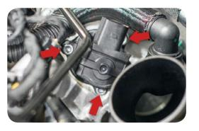
22. Install the DV plug inside the turbo. The plug should sit centered in the opening in the turbo.
