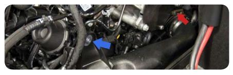
10. Remove the clips attaching the wire harnesses to the factory pipe. Depending on your vehicle there will be either 3 or 4 clips.
