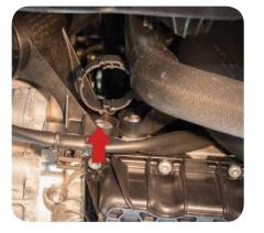
15. Position the outlet pipe allowing proper clearance between the radiator hoses, fans, and shift linkage on top of the transmission. Once positioned properly tighten the 7mm hose clamp at the turbocharger and 8mm clamps between the outlet pipes.
