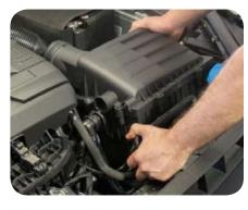
7. Remove the 7mm clamp securing the inlet hose to the turbo.
