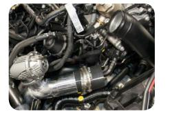
14. From the bottom of the engine bay secure the lower outlet pipe to the block using the supplied allen bolt (red arrow).
