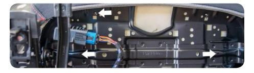
3. With the left side mount points loosely installed open the drawer so the right side mounting hole is exposed. Install the remaining T25 torx screw.
