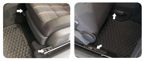
2a. With the bolts removed, carefully tilt the seat backwards so the underside can be exposed. The three included torx screws will secure the drawer to the underside of the seat. The screws will install into the holes shown below. Since the screws will need to form threads as they are tightened we recommend using a drill or impact driver to tighten the screws.
