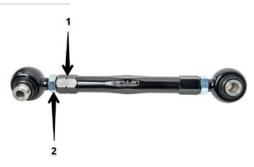
3. Place new control arm and your OEM control arm side by side. Then loosen or tighten center of adjustable control arm until your new control arm is the same length as the original piece. The bolt holes should all line up correctly. Repeat this step with each side.
