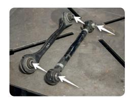
4. After sliding the new Spulen adjustable control arms over the sway bars, place them into factory location. Replace the OEM nuts and bolts at locations 1 and 2. Repeat this step for the opposing side.
