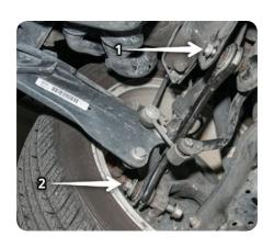
2. Hold center of new control arm at point 1 with a wrench and loosen the lock nut at point 2. Repeat for opposing end of control arm.
