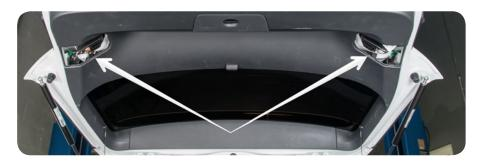
4. Using a razor blade on drivers side plug, cut off protruding tab as shown. Both sides of plug should be flat. Note: this only needs to be done on drivers side plug.
