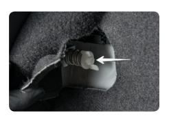
7. Secure new tail lights using OEM 8mm nuts and reconnect harnesses.
