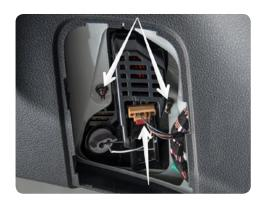
10. Remove tail lights just enough to reach between them and the body of the car. Release red clip then disconnect harness and remove tail lights. Install new tail lights in reverse order.
