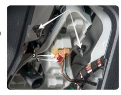
5. Remove hatch lights by first pulling up (1) and then away (2) as shown. Repeat for both sides.
