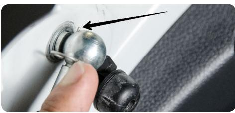
11. Lock the retaining clip into place by rotating it until it clips into the groove on the gas spring. Repeat for both ends of the gas spring.
