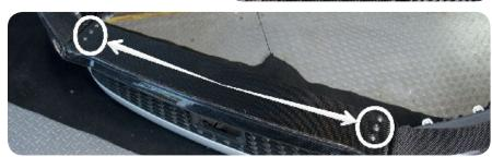
13. Apply pressure inside center of bumper pushing into grille to close any gap. While holding flush, insert self tap screw in underside of grill. Reinstall center diffuser piece to cover this self tap screw.
