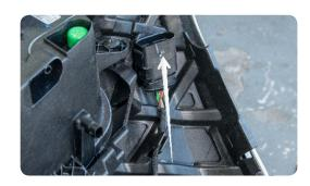
7. Angage clips as shown and remove air scoops.
