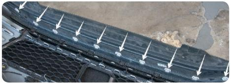
9. Once again starting from one of the ends, pull the grill clips away from the front diffuser one at a time. This will allow the OEM front diffuser to come off. Although this may take one person to pry the clips away as another person pulls the lip out.
