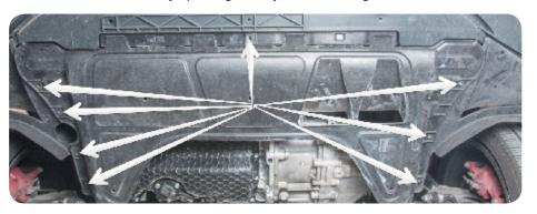
2. Remove two torx screws from side under body splash guard, on each side. Totaling four screws.
