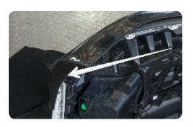
11. Now on the opposing end, apply some force to push the bumper into the front diffuser corner.
