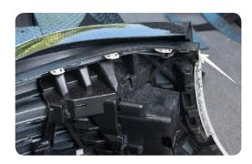
12. Remove 6 allen bolts securing center front piece of diffuser and remove center diffuser piece.
