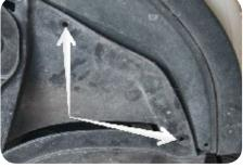
3. Remove two screws from grille (OEM torx or allen keys with USP Clean Bay Bolt Kit)
