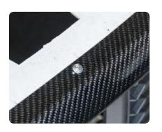
14. Hold diffuser ends flush with bumper and insert two self taps in each side as shown.
