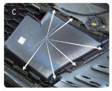
8. Starting from the ends, disengage all clips securing OEM front diffuser.
