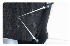
8. Using supplied screws, fasten diffuser onto bumper from below as shown.
