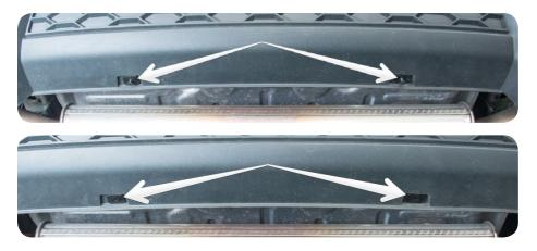
4. Pull back on fender lining and slide out plastic which holds rear diffuser into place, on both sides.
