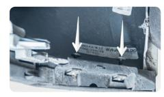
3. Unfasten two plastic screws from rear bumper and remove clips.
