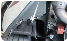
2. Remove two torx screws from inside of each corner of the bumper.
