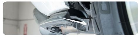
**5.** Disengage all 14 OEM diffuser securing tabs along inside of bumper and remove OEM diffuser.
