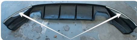
7. Peel back paper liner on double sided tape and hold new Carbon Fiber Rear Diffuser onto bumper carefully. When lined up correctly apply force at double sided tape locations. Then fasten ends onto bumper using supplied screws as shown.
