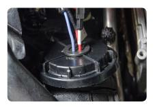
10. Appropriately connect all wires to ballasts as shown.
