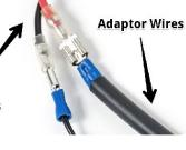
7. Push heat shrink over connectors, and apply slow heat until formed into shape.
