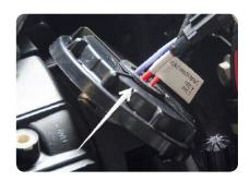
9. When rubber grommet with wires is sealed on plastic cap, fasten cap onto back of head-light housing.
