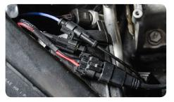
11. Tuck wires underneath headlight and mount ballast where desired using double sided tape.
