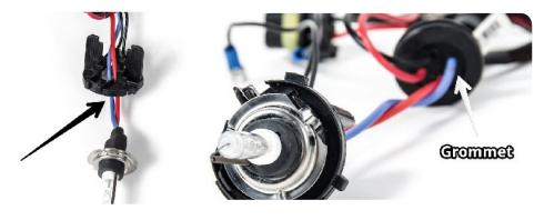
5. Push bulb up against bulb adaptor, with tab resting between two guides on adaptor as shown.
