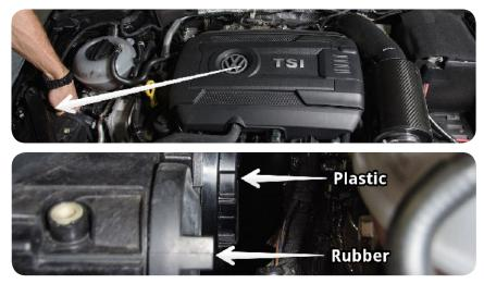
**3**. Drill a 1" hole in the center of this plastic cap.
