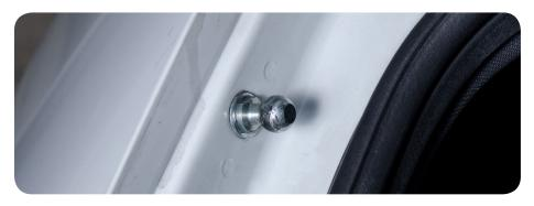
**3.** Apply force on the gas spring away from the base of the ball pin adaptor to disconnect.
