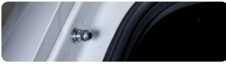
8. Pop the gas springs onto the newly mounted ball pin adaptors. The thicker body of the gas spring with the label, should be mounted on the hatch.
