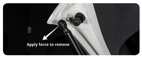
**4**. At the opposite end of the gas spring, use the pick again to disengage retaining clip.
