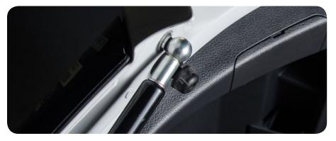
9. Make sure that the ball sockets are centered on the ball pin adaptors.
