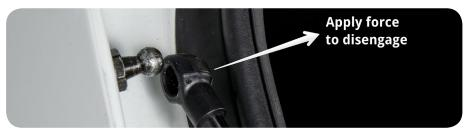
6. Using a 13mm socket and ratchet, remove the original ball pin adaptor from body of car and hatch.
