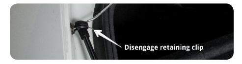
5. Apply force on gas spring away from the base of the ball pin adaptor to disconnect.
