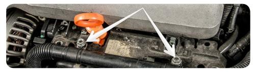
6. Remove the two allen key bolts on this bracket and slide the bracket to the side.
