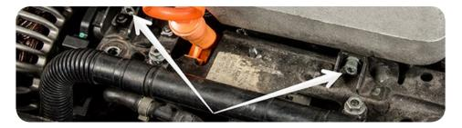
7. Locate the final OEM hose connection which is located below the intake manifold and disconnect.
