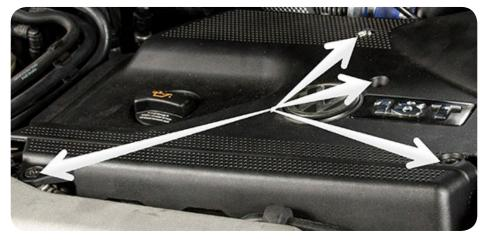
2. Remove the plastic cover in front of the intake manifold by loosening the two securing clips using a flat head screw driver.
