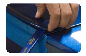
3. Carefully go over your trunk, to remove any double sided tape residue.
