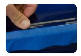
4. Using the supplied double sided tape, run one long strip along the bottom side of the Aggresiv Carbon Fiber Spoiler.
