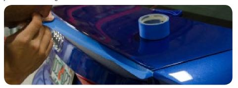
2. Using the wedge tool, carefully pry up on your OEM spoiler releasing the double sided tape. Ensure that the wedge tool is resting on the blue painters tape for leverage. Work your way across the entire spoiler until all the double sided tape has been separated.
