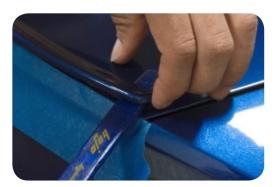
**4**. Using the supplied double sided tape, run one long strip along the bottom side of the Aggresiv Carbon Fiber Spoiler.
