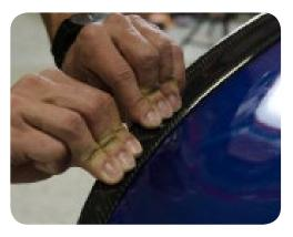
3. Carefully go over your trunk, to remove any double sided tape residue.
