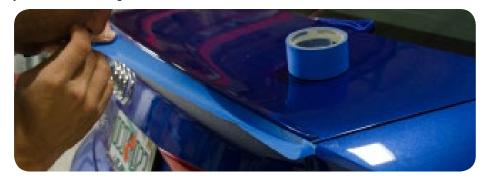
2. Using the wedge tool, carefully pry up on your OEM spoiler releasing the double sided tape. Ensure that the wedge tool is resting on the blue painters tape for leverage. Work your way across the entire spoiler until all the double sided tape has been separated.
