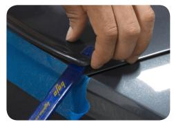
3. Carefully go over your trunk, to remove any double sided tape residue.
