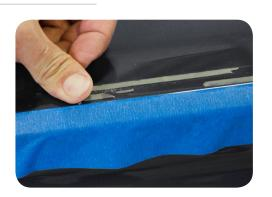
**4**. Using the supplied double sided tape, run one long strip along the bottom side of the Aggresiv Carbon Fiber Spoiler.
