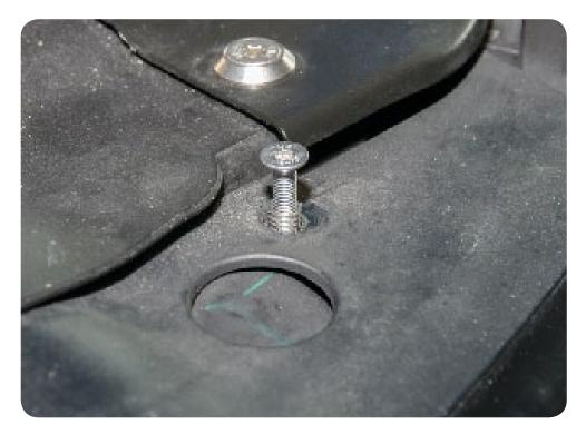
6. Remove screw, and make sure insert is flush with plastic. Reinstall screw using washer (B1), gently threading into insert until snug. Once snug, turn another 90 degrees to secure (use caution not to use excessive torque on these screws).
