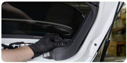
7a. Using a T25, remove the (4) screws holding in the trim piece on the hatch.
