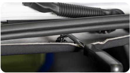
5. Using the wedge tool on the passenger side only. Pop out the bottom side of the hatch wiring loom grommet by pressing in on the tab and then pushing upwards. Pop out the top grommet by pressing in on the tab and then pushing downwards. Be careful not to use too much force or you may break the tab.
