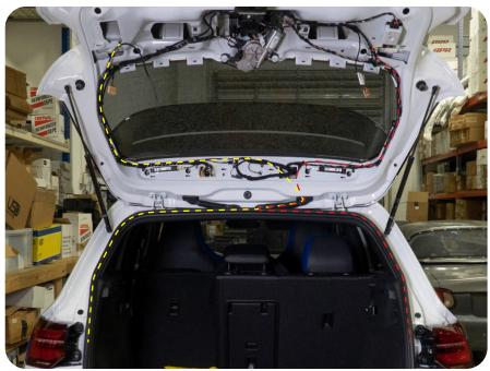
15. Connect the female plug on the harness into the male end on the vehicle harness and the male plug into the tail light. Repeat for the other side.
