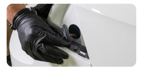
11. Using a tool as a wedge for your fingers, carefully pull back on the liner until you disconnect the liner from these (3) metal tabs.
