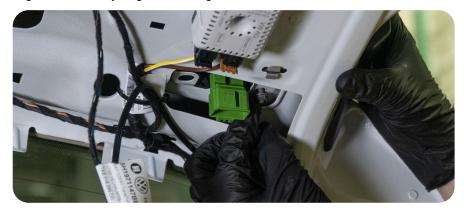
18. Connect the associated taps together. Taps 1 - 1, 2 - 2, and 3 - 3. Then connect the blue female plug from the USP harness into the brown male plug from the vehicle. Repeat for the other side.
