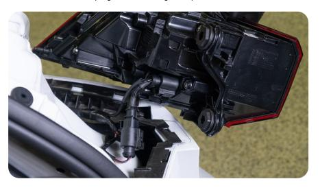
16. Re-install the tail lights using the (2) T25 Bolts. NOTE: After completing the installation, you will need to tighten and align as necessary to get the tail light to sit flush with the hatch. Repeat for the other side.
