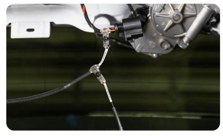
21. Reinstall all of the trim pieces removed by reversing steps 6 and 7. Reconnect both ends of the hatch wiring loom weather cover from step 5.
