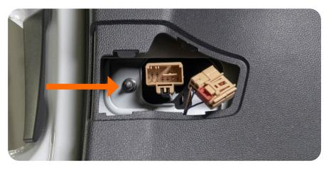
3b. Remove the tail light by pushing upwards and out.
