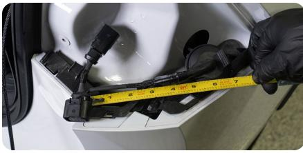
13. Simply feed the harness into the cab. If needed use a guide to help route the wire straight through. Once the harness is fully passed into the cab reinstall the outer weather grommet.
