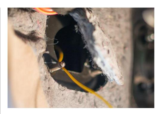
B. IF THE VEHICLE IS MANUAL, YOU WILL NEED TO ROUTE THE WIRE THROUGH THE FACTORY WIRE HARNESS GROMMET TO THE LEFT OF THE CLUTCH PEDAL.
