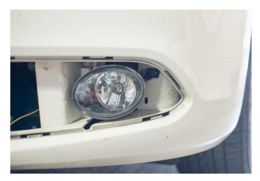
12. Install the supplied fog light grill. Starting from the outer side of the bumper, pop the grill into place making sure the locking tabs clip into the bumper.
