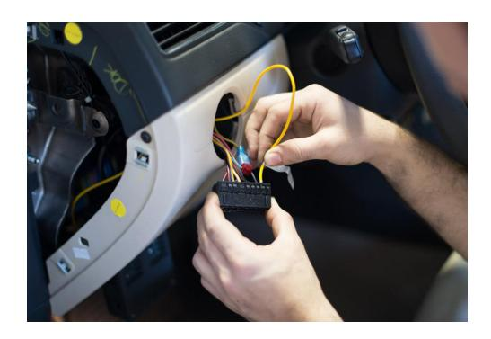
19. CONNECT THE HARNESS TO THE INCLUDED HEADLIGHT SWITCH AND PRESS THE SWITCH BACK INTO PLACE. IF YOU CURRENTLY HAVE THE RFB AUTOMATIC HEADLIGHT CONVERSION, THE INCLUDED SWITCH WILL NOT BE USED.
