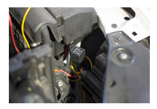
14. CONNECT THE RED WIRE FROM THE WIRE HARNESS TO THE POSITIVE TERMINAL OF THE BATTERY AND THE BROWN WIRE TO THE NEGATIVE TERMINAL.
