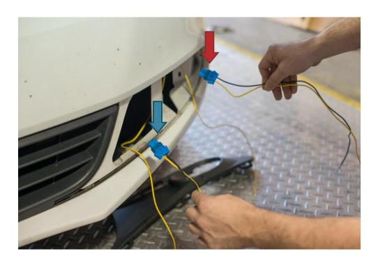
4. THE LONGER LEAD FROM STEP 3 WILL NEED TO BE ROUTED TO THE HOLE IN THE PASSENGER SIDE OF THE FRONT BUMPER. ROUTE THE LEAD THROUGH THE LOWER FRONT GRILL AND TUCK THE WIRES INTO THE BUMPER.
