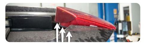
7. Make sure to drop the wiring inside the trunk safely before mounting your new LED lights.
