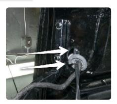
21. Run the new harness into the center of the grommet and pop the grommet carefully back into place.
