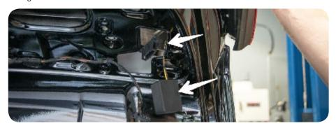
8. Begin mounting the lights by dropping them in at the same angle that the OEM lights were removed. Make sure the black plastic slides over the metal edge of the trunk as shown.
