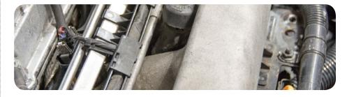
10. Connect the black clip from the tail light to the factory wire harness. connect the white clip from the tail light to the white clip from the supplied wiring harness.
