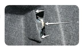
14. Behind the small door, loosen the plastic wing screw which holds the lower tail light in place.
