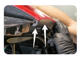
9. Once the tail light has slid from an angle into place over the edge of the trunk, it can be dropped straight into position. tighten the two factory 11mm nuts to secure the new tail lights into place. this will also pull the light in flush with the trunk lid.
