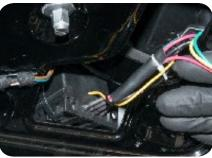
12. Run the new wiring harness down behind the trunk arm, and secure it using wire ties. Leave the wire end hanging, we will return to this in a later step.
