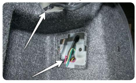
17. Connect the factory harness to the new tail lights as well as the new harness. Replace the new tail light and secure using the OEM plastic wing screw. Then put the small door back into place.
