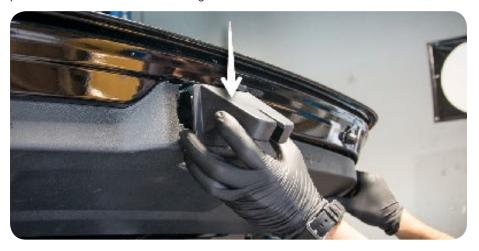
**4.** After you have removed the cover, there are (4) 11mm nuts holding the taillights in place. Only remove the nuts from one tail light at a time, leaving the opposing tail light safely in place for the moment.
