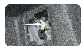
15. Remove the tail light gently just enough to reach behind it. Push in the ends of the clip and remove the connector allowing you to completely remove the factory lights.
