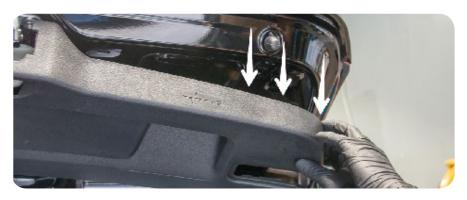
**3.** Once half of the interior cover from the lid has been loosened, remove the plastic shroud on the trunk locking mechanism.
