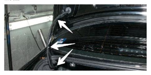
23. Feed the end of the wiring harness behind the trunk paneling and clip the trunk arm plastic cover back into place.
