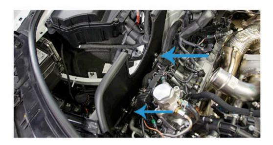
16. Install one of the supplied silicone couplers along with a 2.25" and a 2.5" hose clamp onto the passenger side turbo inlet pipe. Do not tighten the hose clamps at this point.
