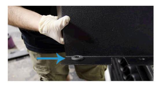
10. Install the driver side heat shield by sliding the rubber grommet onto the post (red arrow). Install the supplied 19mm bolt into the threaded hole in the frame rail (blue arrow).
