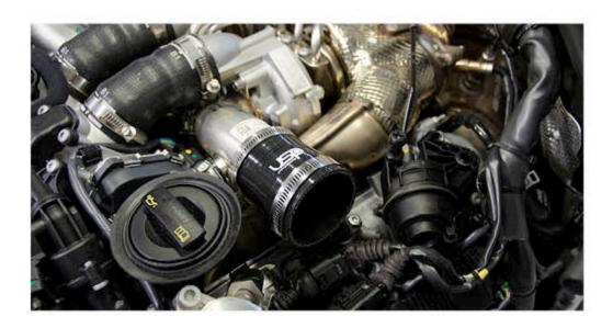
12. INSTALL ONE OF THE SUPPLIED AIR FILTERS ONTO THE DRIVER SIDE INTAKE PIPE. DO NOT TIGHTEN THE HOSE CLAMP AT THIS POINT.
