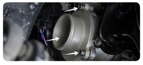
**13**. Install Spulen coupler with logo facing up as shown. This will be a good starting point but may require some rotation of the coupler for perfect fitment with pipe. Install supplied clamps and fasten on turbo muffler delete.
