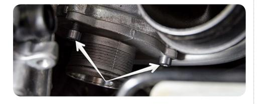
11. Ensure that the O-Ring on the turbo stays in the original groove. If the O-Ring falls out, or does not stay in place use a small amount of grease to hold it in place.
