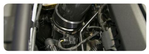
8. Remove the T-30 screw (blue arrow) and loosen the 7mm hose clamp (red arrow).
