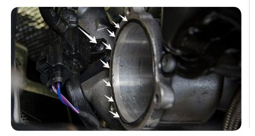
12. Install the included O-Ring into the groove on the smaller end of the turbo muffler delete. If it is not staying in the groove, use a small amount of grease to ensure the O-Ring does not fall out. Then install the turbo muffler delete and secure using the (3) factory allen key bolts.
