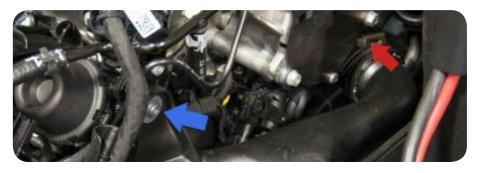
9. Loosen the 7mm clamp and slide the turbo outlet pipe to the side enough to remove the rubbber coupler and acceess the OEM turbo muffler
