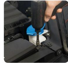
2. Remove the coolant line from the front intake snorkel.
