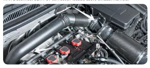
2. Remove T25 torx screw securing OEM intake to exhaust manifold heat shield.
