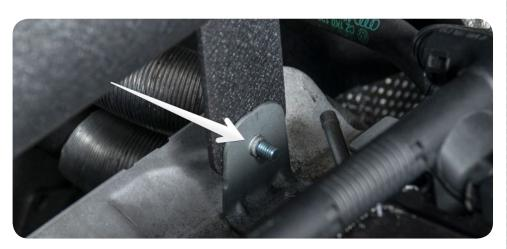
7. Secure two remaining clamps at MAF connection.
