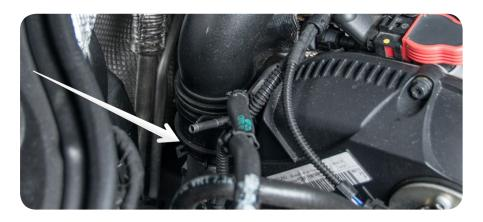
4. Place silicone reducer on end with PCV fitting and straight silicone on opposite end. Then drop intake into place. First connection to be made is the PCV hose, which clips onto machined lip.
