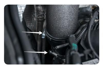
**6.** Install supplied fastener into bracket while supporting intake from not resting on brake fluid reservoir.
