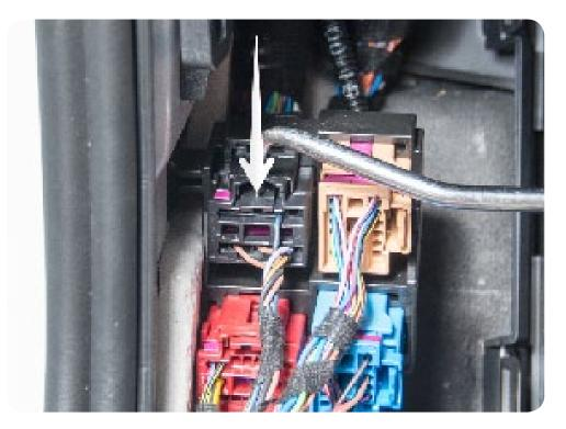
12. Turning the connector upside down (connector securing tab is now facing down), insert supplied wire pin into slot 5 as shown.
