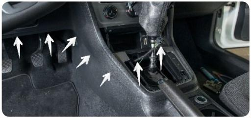
**15**. Run harness into slotted area and connect to new traction control switch.
