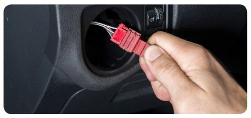
10. Connect male end of jumper harness into headlight switch. Then feed jumper harness into dash and down towards footwell.
