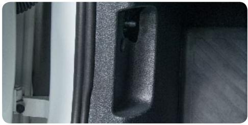
6. Loosen lower kick panel by pulling up at the front, allowing to slide front portion to the side in order to access front kick panel.
