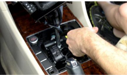
4. REMOVE THE CENTER CONSOLE BY PULLING UPWARDS.
