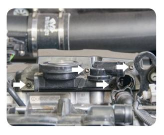
4. Install the Spulen PCV plate using the factory T-25 screws. Make sure the fitting on the adapter plate is tight. Reattach the lower breather hose.
