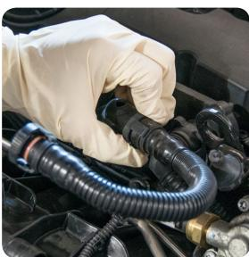
2. Remove the hose that connects the lower breather hose to the PCV valve.
