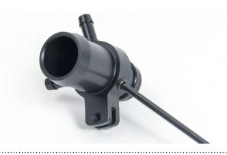
6. Lightly coat the threads of the included 6mm plug with thread lock and install into center of boost tap.
