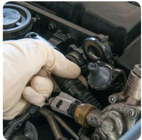
3. Remove the 4 T-25 torx screws securing the PCV valve to the valve cover.
